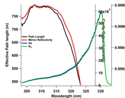
Spectra were fitting using a custom Python fitting algorithm. A sample fit is shown at left.
