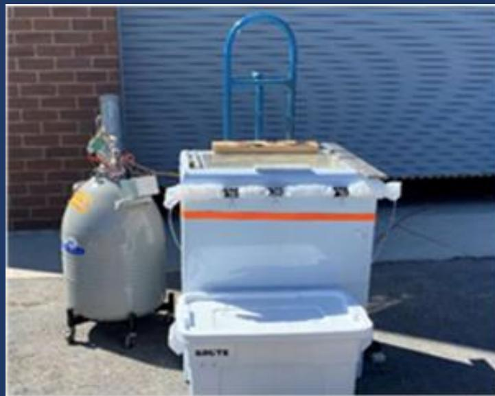
Figure 3: Photograph of modified freezer and liquid nitrogen apparatus that maintained temperature within freezer in the presence of natural sunlight.
