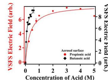
Figure 8. VSFS electric fields of  $-\text{CH}_2\text{-as}$  as a function of butanoic acid concentration in 0.5 M NaCl seed solution (black solid diamond, right axis), in comparison with those for propionic acid (red solid circle, left axis). Error bars represent 5% deviation.
