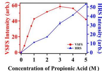
Figure 5. VSFS (red solid circle, left axis) and HRS (blue solid triangle, right axis) intensities at 2991.8  $\text{cm}^{-1}$  ( $\text{CH}_2\text{-as}$ ) as a function of propionic acid concentrations added. Error bars represent 5% deviation.
