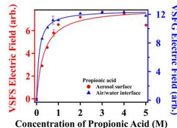
Figure 7. VSFS electric fields of  $\text{CH}_2\text{-as}$  for aerosol curved surfaces (red solid circle, right axis) and VSFG electric fields of  $\text{CH}_2\text{-as}$  for the air/water planar interface (blue solid triangle, right axis) as a function of propionic acid concentration in a 0.5 M NaCl seed solution. Error bars represent 5% deviation.
