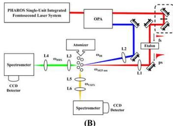
Figure 3. A) A schematic diagram of the beam management in VSFS experiments. A picosecond 1025 nm and a broadband IR light were non-collinearly incident on samples. B) Schematic diagram of both the VSFS and HRS experiments. A spectrally narrow picosecond 1025 nm from an etalon was combined with a broadband OPA-generated IR femtosecond pulse at the aerosol samples to yield sum-frequency and hyper-Raman signals.
