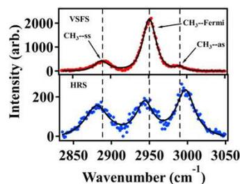
Figure 4. HHH-polarized configuration spectra for VSFS (upper) and HRS (lower) for aerosol particles from a 0.5 M NaCl seed solution with 4.0 M propionic acid.
