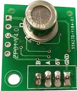
Ozone sensor: <https://www.winsen-sensor.com/sensors/o3-gas-sensor/ze27-o3.html>
