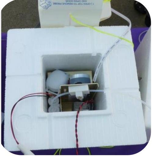
(left) The Ozonesonde, or ozone-detector, is like a small chemical laboratory. It has a small pump which takes in surrounding air and passes it through two chambers of chemicals. If ozone is present, the chemicals react, creating a potential cell that outputs direct current. The level of the current is transmitted to the ground station as data to be collected.
