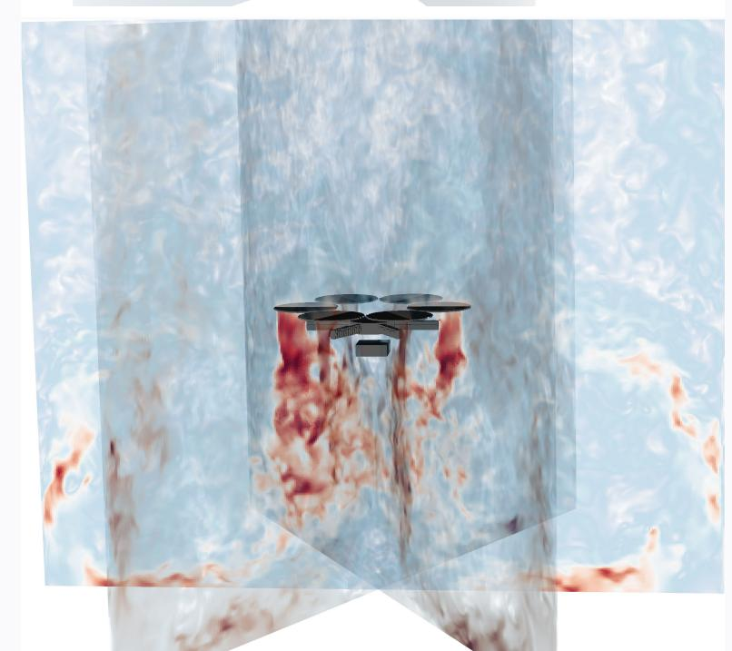
Fig. 3: Airflow (m/s) during ascent (top) and descent (bottom)
