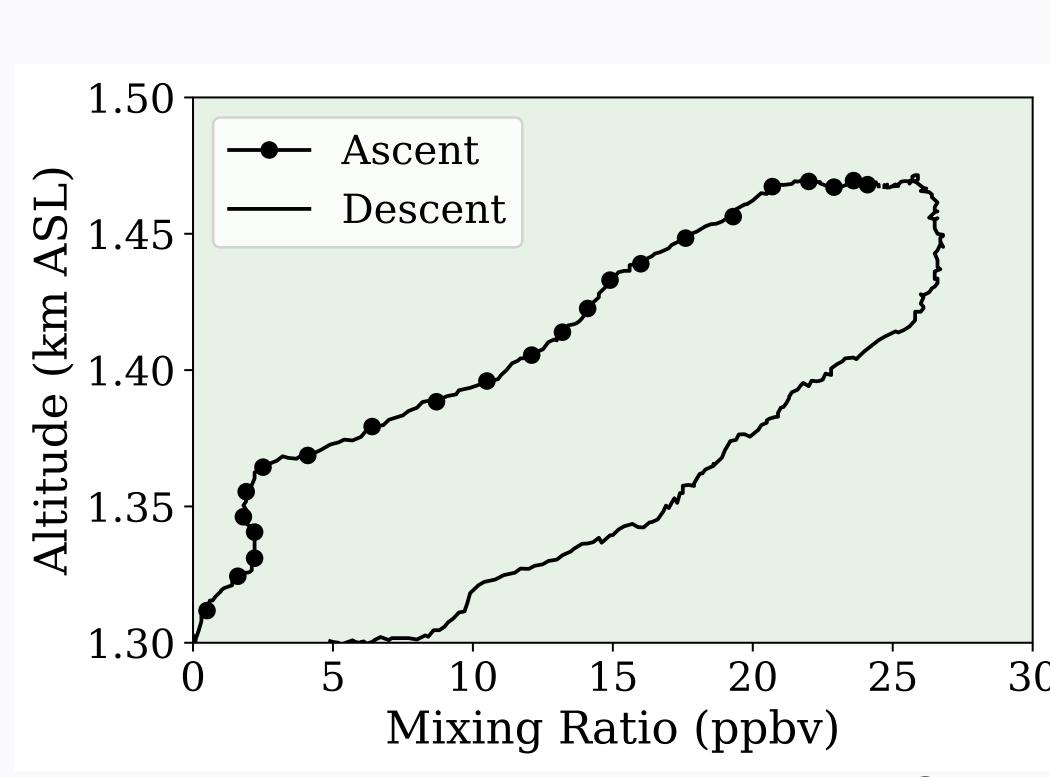
Fig. 2: Morning ozone profiles measured during ascent (dotted line) and descent (solid line)
